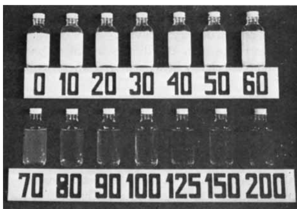
Fig. 9. Optical density changes undergone by latex EA/MAA, 80/20, 0.5% BTCM, at stated degrees of neutralization (2.0% polymer solids).
